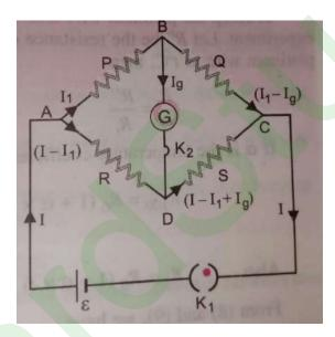
For four resistances P,Q, R and S, the Wheatstone Bridge is said to be balanced when:
