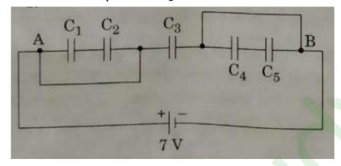
As the combination of  $C_1$  and  $C_3$  and  $C_4$  and  $C_5$  are shorted.
