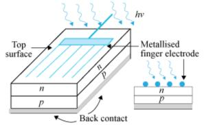
It generates emf when solar radiation fall on the p-n junction. A p-type silicon wafer of about 300  $\mu$ m is taken over which a thin layer of n-type silicon is grown on one side by diffusion process.
