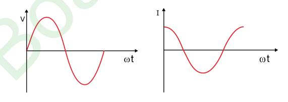
Phase relationship between  $\omega$  and I On comparing equation (1) and (2), we find that in a capacitive a.c. circuit, the current leads the voltage or the voltage lags behind the current in phase by  $\pi/2$  radian. The phase relationship between v and I is shown graphically in Fig.(a). We see that the current reaches its maximum value earlier than the voltage by one-fourth of a period.
