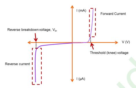
When a p-n junction diode is reverse biased, minority charge carriers of the diode drift across the junction towards the ends of the diode. The movement of these minority charge carriers produces currents of very small value. At any temperature, the number of minority charge carriers is constant. So the current flow due to these charge carriers also remains constant and it is independent of any applied potential difference.
