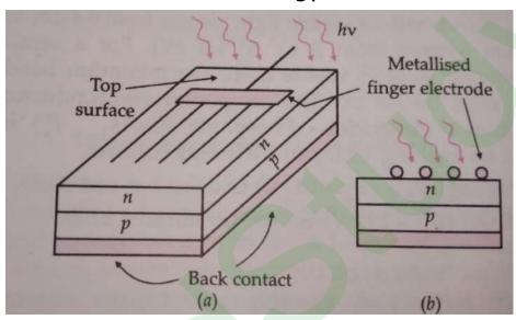
Here fig. (a) represents a typical p-n junction solar cell and fig. (b) represents the sectional view of the same solar cell.
