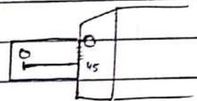
$$\begin{aligned} \text{-ve zero error} &= -\text{LC} \times \text{coim. div.} \\ &= -(0.01) \times 5 \\ &= -0.05 \text{ mm} \end{aligned}$$
