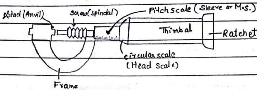
Pitch  $\Rightarrow$  The distance covered by screw in one complete rotation of the circular scale is called pitch.
