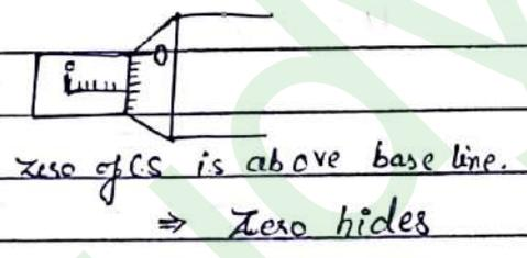
$$\text{Correct Reading} = \text{Reading} - \text{Zero error}$$
