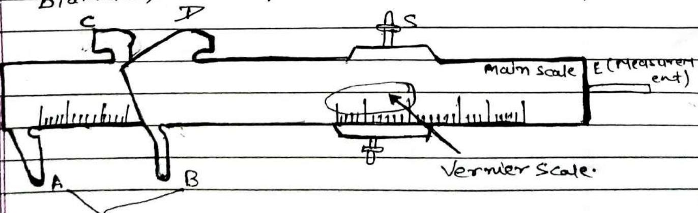
Jaws (measure diameter of small cylindrical body).
