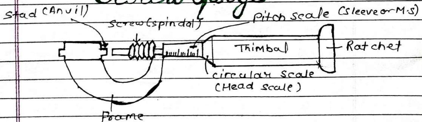
Pitch  $\Rightarrow$  The distance covered by screw in one complete rotation of the circular scale is called pitch.
