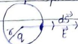
$\vec{E}$  and  $d\vec{s}$  at any point on  $S$  are directed radially outward.
